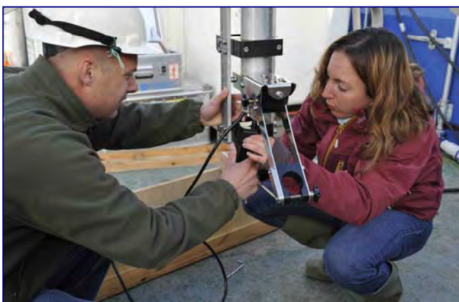
Dick and Cecile Cathalot mount the instruments on the "Eddy covariance" lander (above) before it is deployed at 280m depth in the Træna coral field (right). It gives an estimate of oxygen uptake by the benthic habitat without taking a sample of the bottom. The lander is about 1.5m high.
