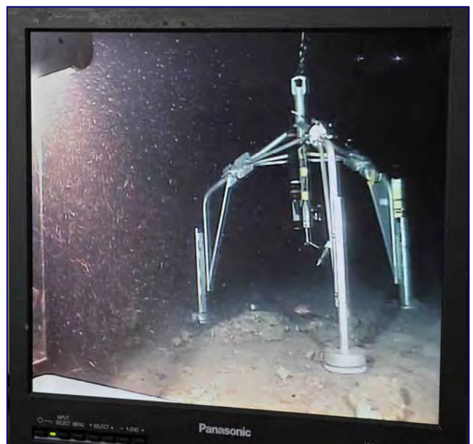
Dick and Cecile Cathalot mount the instruments on the "Eddy covariance" lander (above) before it is deployed at 280m depth in the Træna coral field (right). It gives an estimate of oxygen uptake by the benthic habitat without taking a sample of the bottom. The lander is about 1.5m high.
