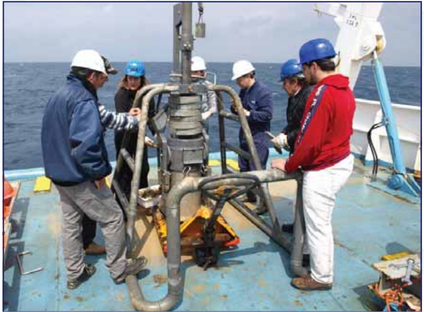
The box-corer on deck. Chief Scientist Dr Alessandra Savini is in the light blue hat.
