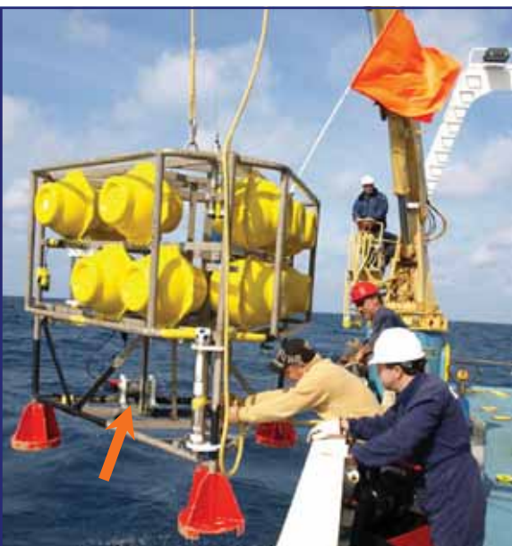
The NIOZ lander being retrieved after a successful deployment. The camera is indicated by the arrow, and the yellow spheres are the floats.
